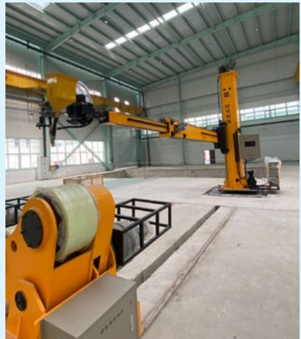
Welding manipulator with boom inner extension
