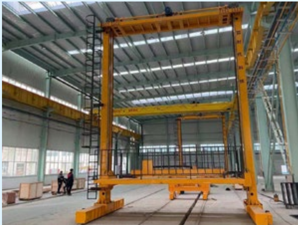
Gantry welding manipulator
