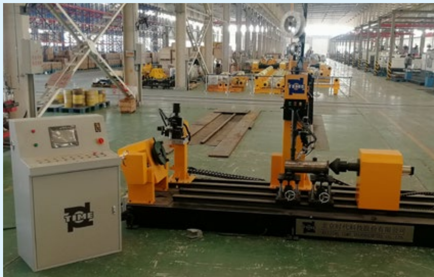
Welding equipment of horizontal longitudinal seam, vertical circumferential seam, small TDMAW welding
