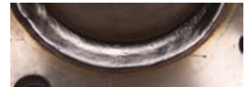
Stainless steel MIG flux-cored wire Current: 270A Voltage: 27.7V
