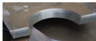
Carbon steel Cutting current: 260A
