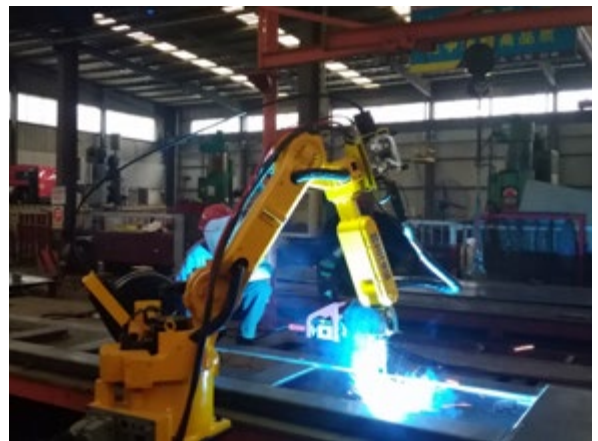
Welding of carriage plate
