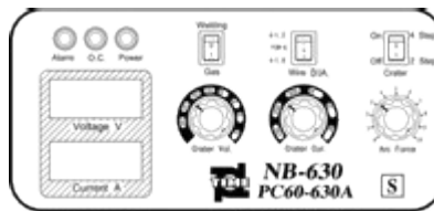
Carbon steel MIG horizontal position Current: 140A ~ 160A Voltage: 21.5V ~ 23V
